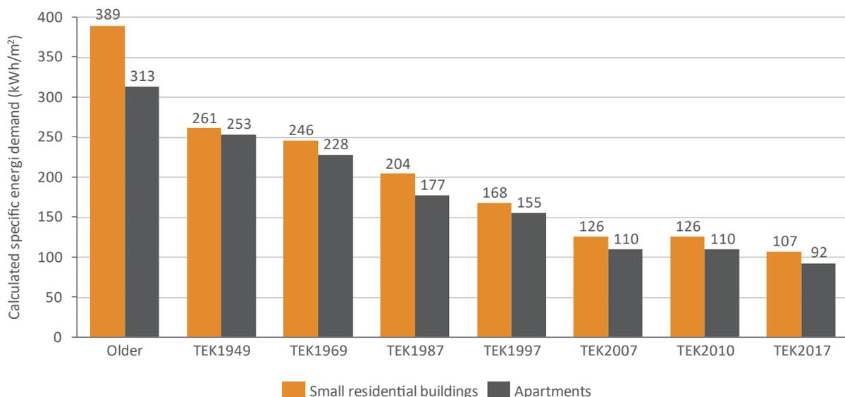
Figure 3 Development in calculated specific net energy demand based on building code and building tradition. (Source: Multiconsult, simulated in SIMIEN)
