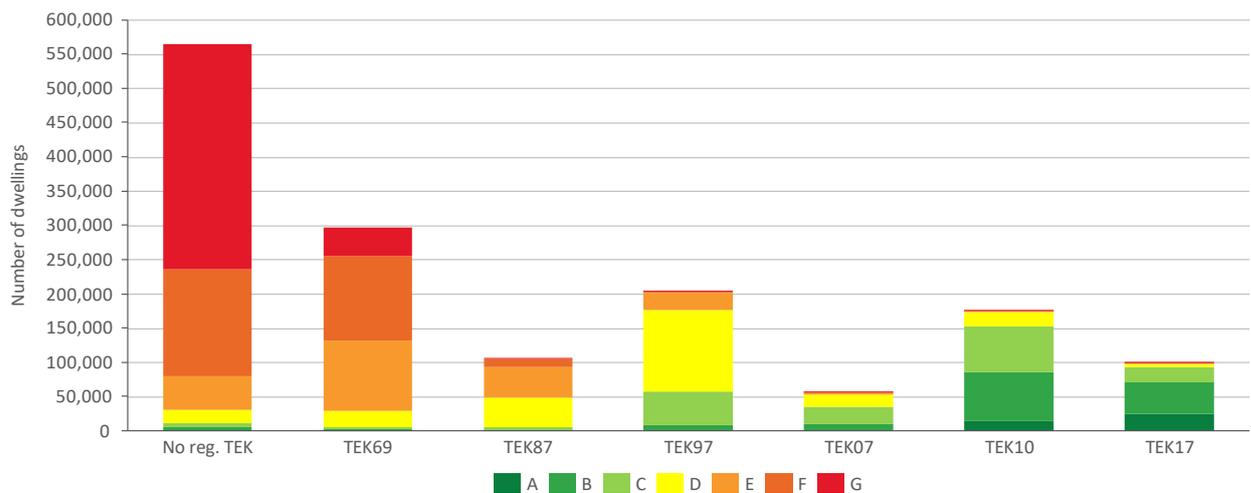
Figure 5 Registered EPC Certificates Norwegian residences distributed per building code and Energy Performance Certificate. (Source: EPC database, [energimerking.no](http://energimerking.no) January 2023, [enova.no/energimerking](http://enova.no/energimerking) February 2024).
