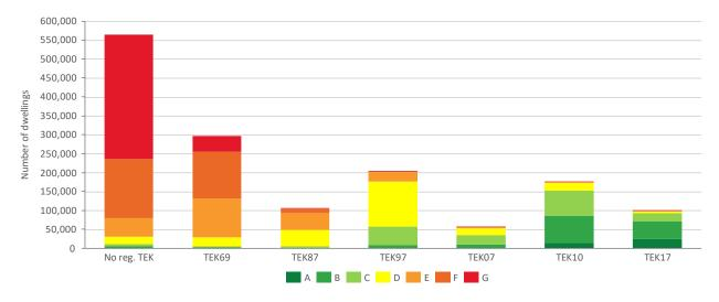
Figure 5 Registered EPC Certificates Norwegian residences distributed per building code and Energy Performance Certificate. (Source: EPC database, energimerking.no January 2023, enova.no/energimerking February 2024).
