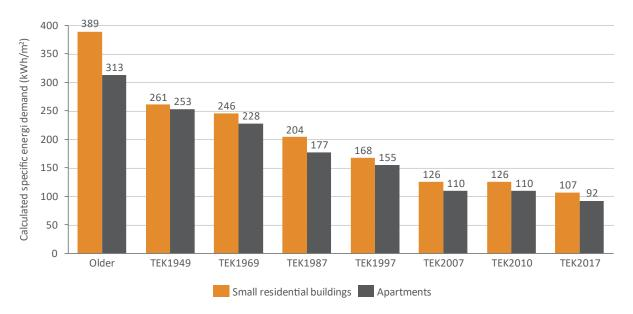
Figure 3 Development in calculated specific net energy demand based on building code and building tradition. (Source: Multiconsult, simulated in SIMIEN)
